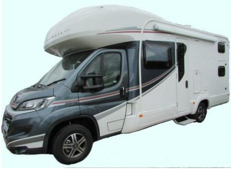
The Auto-Trail Tribute coach-built Hi-Line Model T726 6 berth with rear bunks/garage is a luxury Fiat Ducato based motor home with a 130bhp turbo diesel and 6 speed manual gearbox, that any driver could get used to. To complement this it has ABS brakes, cruise control, cab air conditioning and power steering.
